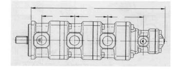
Quadruple pump assembled from 3 different frame sizes
