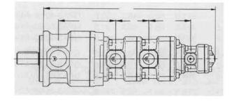
Quadruple pump assembled from 2 different frame sizes
