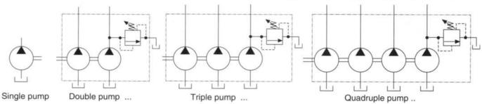
... equipped with pressure relief valve (optional) for cover end pump section and external tank port
